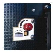
Adjustable brush speed means that the machine can deal with all road surfaces and dust conditions (optional)
