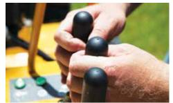
**OPERATOR PRESENCE SYSTEM.** Control handles for the boom swing, boom raise/lower and machine propel are equipped with an operator presence handle design which provides capacitance sensing capability. This user-friendly operator presence system is intended to help protect the operator and enhance operator safety.
