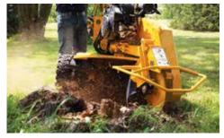
AUTOSWEEP® SYSTEM. When equipped, the AutoSweep function monitors engine speed and automatically adjusts cutter wheel sweep rate, and is designed to reduce engine, drivetrain and structural stress.
