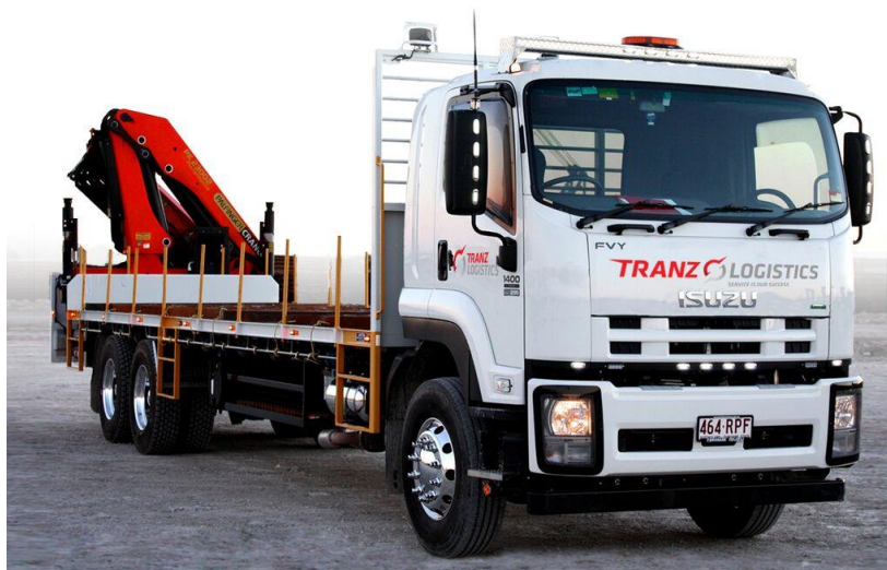
Flatdeck Crane Truck with 9m Tray Front Fitted - PK 23002 EH Palfinger Crane – Max 6,200kgs (See Below)
