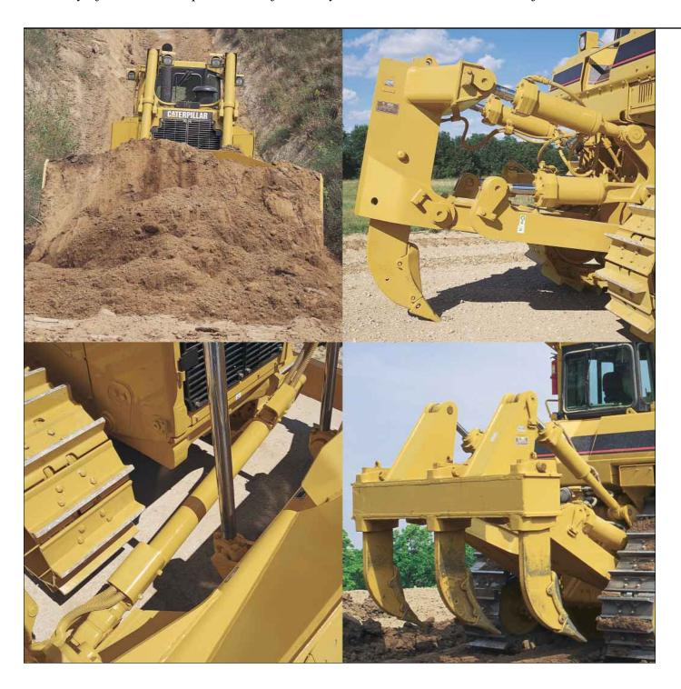
**Blades.** The Universal (U) blade and the Semi-universal (SU) blade make full use of the D8R II power. The U blade has increased capacity and less spillage. The SU blade is built for tough applications in tightly packed material where penetration is more important than capacity.
