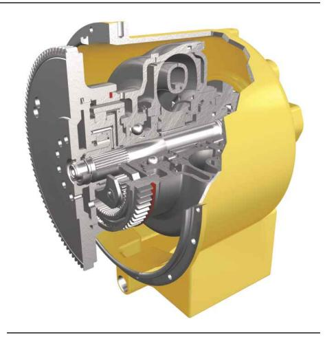
**Freewheel Stator.** Improves torque divider efficiency. During machine operation under low drawbar loads, the stator is permitted to rotate to achieve peak efficiency. The result is a reduction in heat and an increase in fuel efficiency.
