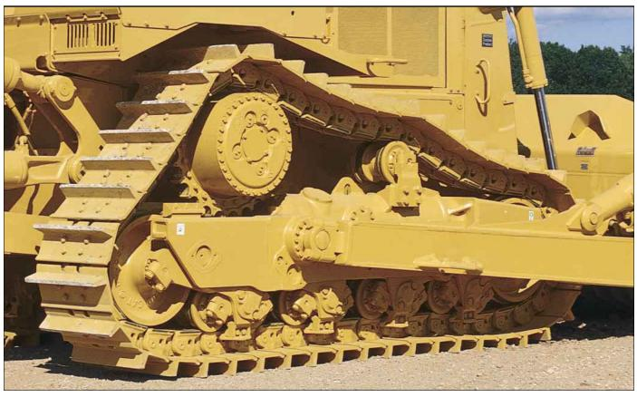
**Bogie Suspension.** Conforms more closely to the ground to provide more ground contact, especially in hard, uneven terrain. Higher traction means less slippage, better balance, and a smoother ride.
