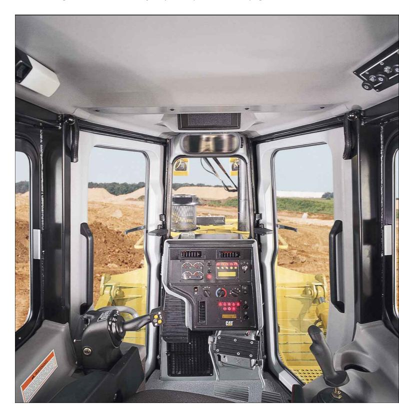
Caterpillar Monitoring System. Provides the operator instant feedback on the condition of operating systems and records such performance data as high/low gauge readings to help diagnose problems and manage undercarriage. Caterpillar Monitoring System provides gauges that monitor the temperature of the engine coolant, hydraulic oil and power train oil, plus the fuel level.
