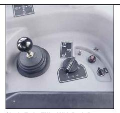
**Single Twist Tiller With Push-Button Speed Control.** New on the D8R II is a single twist tiller with push-button speed controls allowing one-hand control of the direction and degree of turns, forward-reverse shifting, and gear selection.
