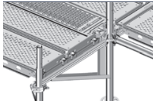
Assembly situation: U-console bracket, 0.73 m wide 3 (top) or alternatively U-ledger 0.73 m in conjunction with Bracket brace 2.05 m 9 (left).
