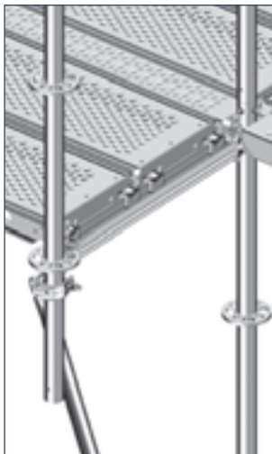
Assembly situation: U-console bracket, 0.73 m wide 3 (top) or alternatively U-ledger 0.73 m in conjunction with Bracket brace 2.05 m 9 (left).
