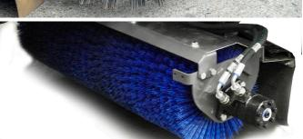
Trailed, robust, steel suction nozzle for durability. Complete with trailed side brush, widesweep brush and optional front brush assemblies all fitted with water nozzles for dust suppresion.
