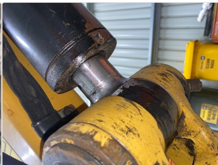
MINOR OIL LEAK @ BUCKET CYLINDER / LINKAGE AREA
