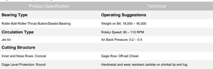
Based on the IADC Bit Classification System located in the IADC Drilling Manual, 11th Ed. – Redesigned, 2007
